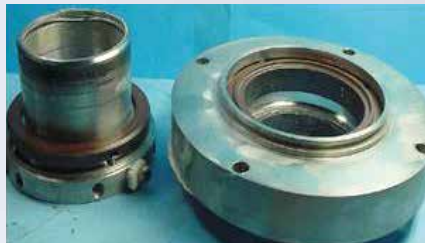
The PowderAce after 4 years of use: After a routine reworking of the sliding faces, the seal was reinstalled.
